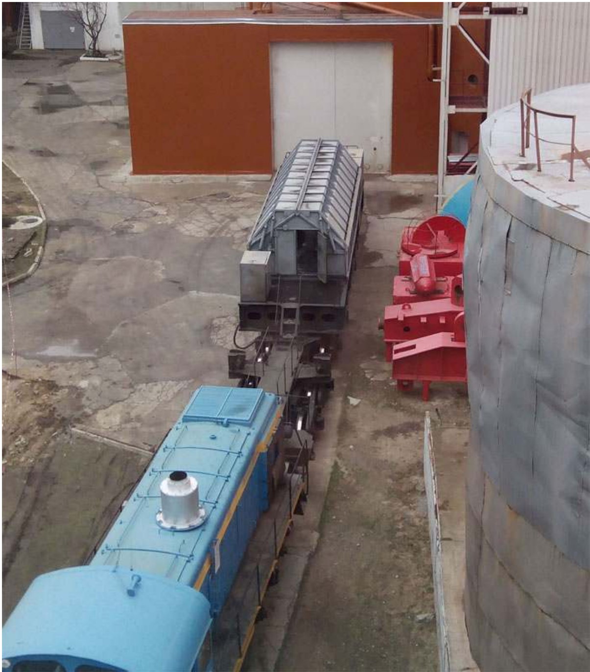
Railway wagon for nuclear fuel transport
