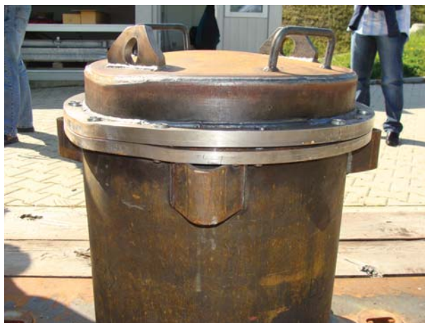
Figure 11.6. Damage after drop
