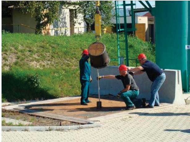
Figure 11.3. Free fall from a height of 1.2 m
