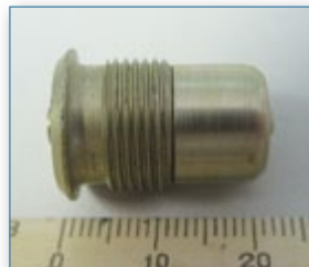
Detected capsule with plutonium used for smoke indicator powering
