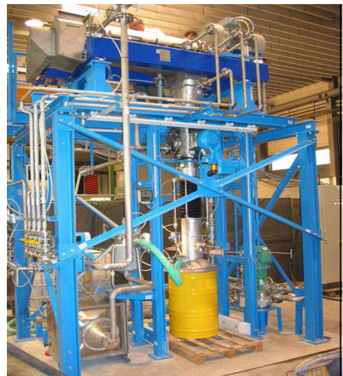
Photo 4. Installation for centrifugation and purification of radioactive oil at RNPP
