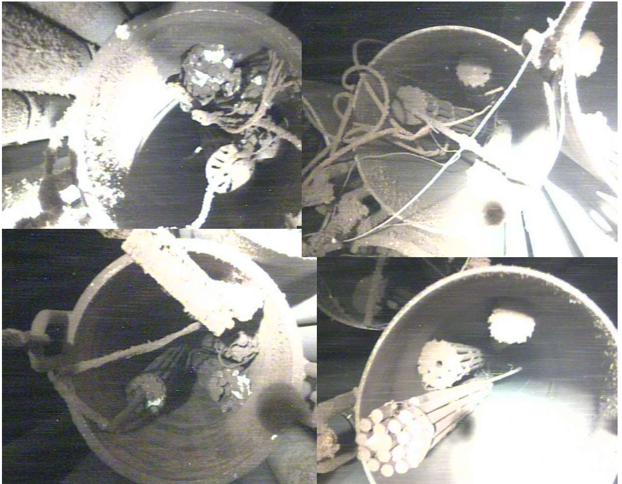
Figure 8.1 – Damaged spent fuel in special canisters
